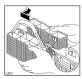
The cutlery basket is in two parts which can be separated to give greater loading flexibility. To separate the two parts, slide them horizontally in opposite directions and pull them apart. To reassemble, reverse the procedure.
